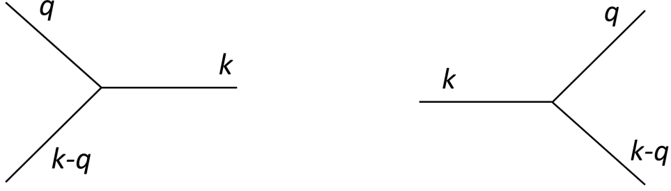
Figure 3.7: Magnon fusion (left) and decay (right) processes induced by spin non-collinearity. Such processes limit magnon lifetime and thermal conductivity.
